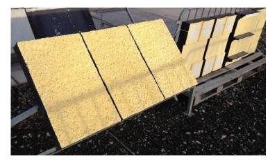
**Figure 2.** Samples with 6 cm aerogel-based render and 3 different finishing coats weather exposed at an angle of 135° at the R&D of Fixit Group in Röthis (Austria).
