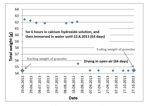
**Figure 5.** Measured total weight for aerogel granules in a metallic net bag immersed in water after a preliminary treatment of 6 h in calcium hydroxide solution with pH > 13.
