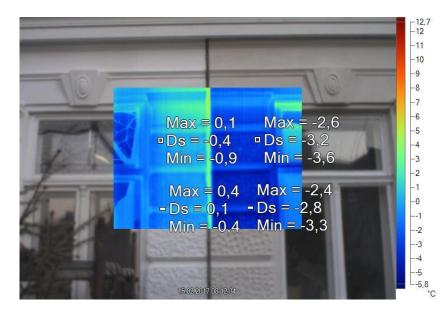
**Figure 9.** The original façade (**left**) and the retrofitted one (**right**) with an infrared inlay in the centre taken at 8 in the morning of 15 February 2017 (min, Max and Ds represent the maximum, minimum and average Temperature in the small square).
