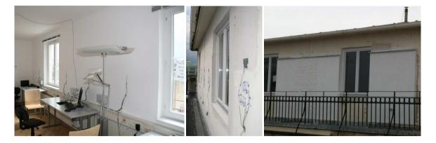
Fig. 1. Position of the temperature and humidity sensors (a) internal surface; (b) external surface prior to retrofit; (c) on the F222 plaster beneath the finish (not visible) after retrofit
